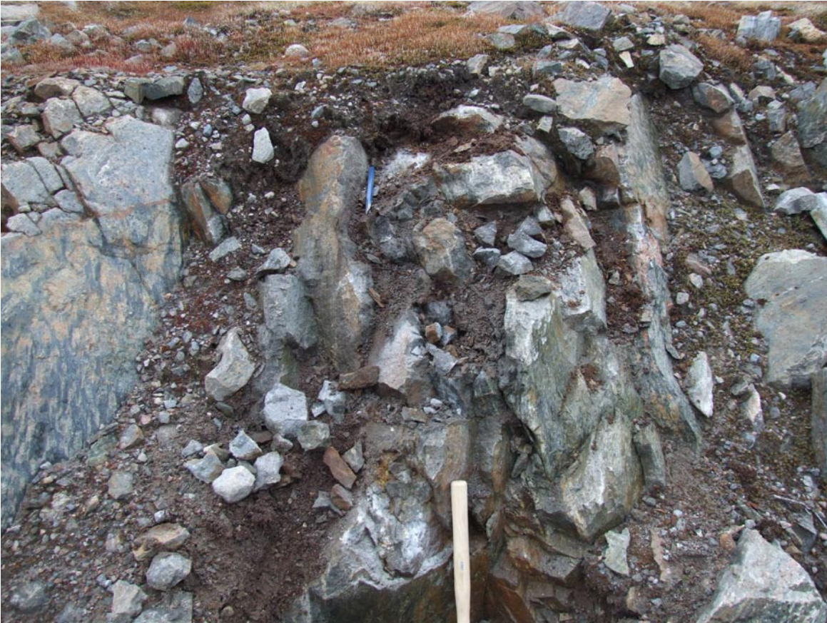
Figure 5. Close-up view of copper-gold showing returning 2.17% Cu and 556 ppb Au.
