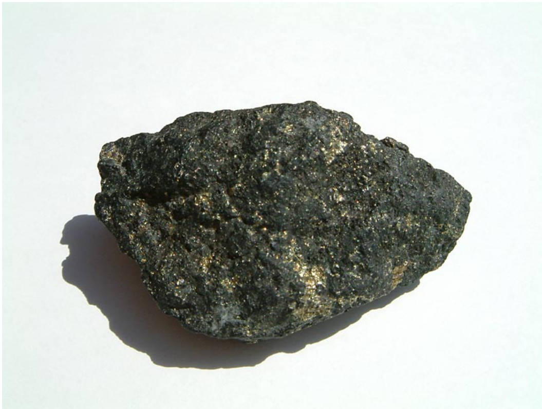
Figure 3. Mineralized sample from a sub-crop on the Labrador Claims. The rock appears to be a gabbro filled with chalcopyrite (Cu-rich), bornite (Cu-rich), and pyrite (Fe-rich).
